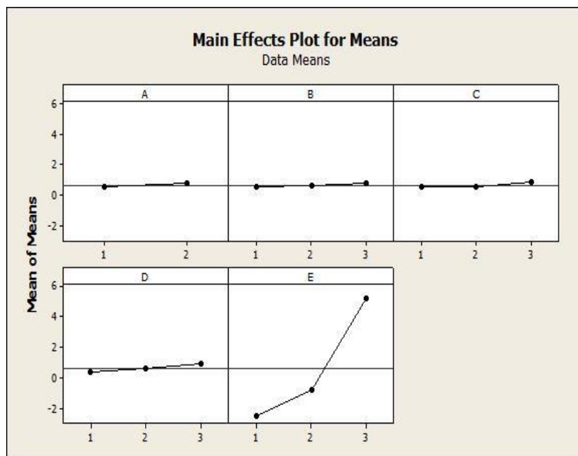
Figure 8 Effect of various process parameters on weld line movement
