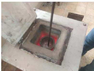
Fig. 1 Stir Casting Furnace
