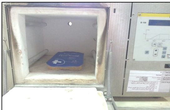
Figure 6. Hot thermal bag in the oven.
