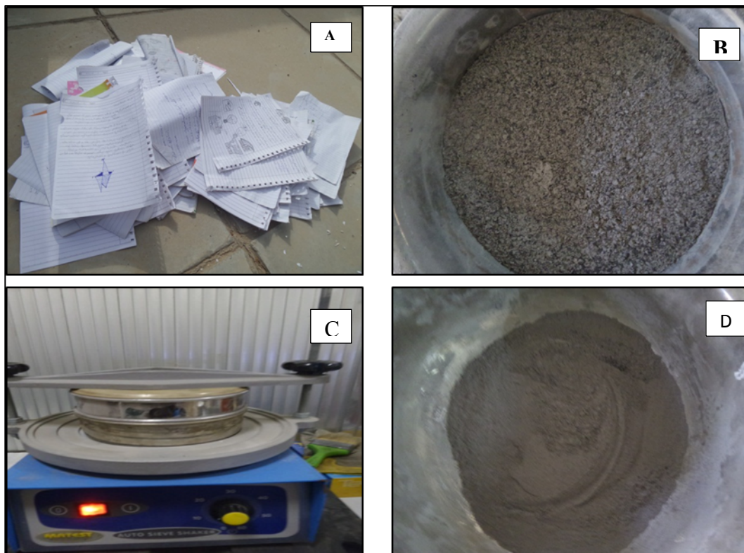
Figure 1. preparation of wastepaper ash (a) wastepaper before burning (b) wastepaper after burning, (c) sieving No,600µm of wastepaper ash, (d) ash wastepaper
