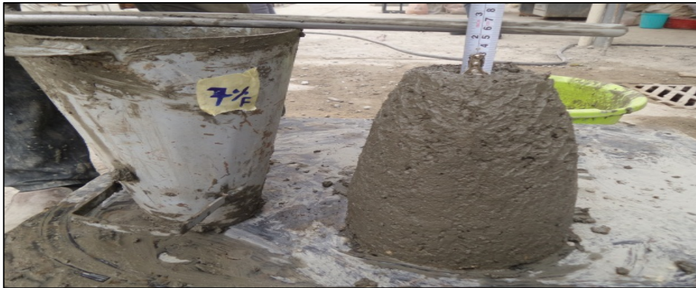
Figure 2. Slump Test
