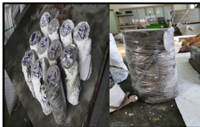
Figure 2. Two similar sections of cement mortar after casting at room temp.
