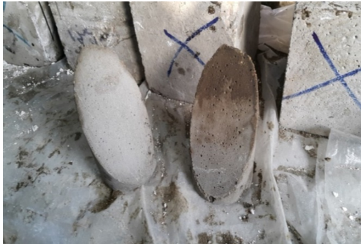
Figure 1. Two similar sections of (150 by 75 –mm) Portland– cement mortar cylinder
