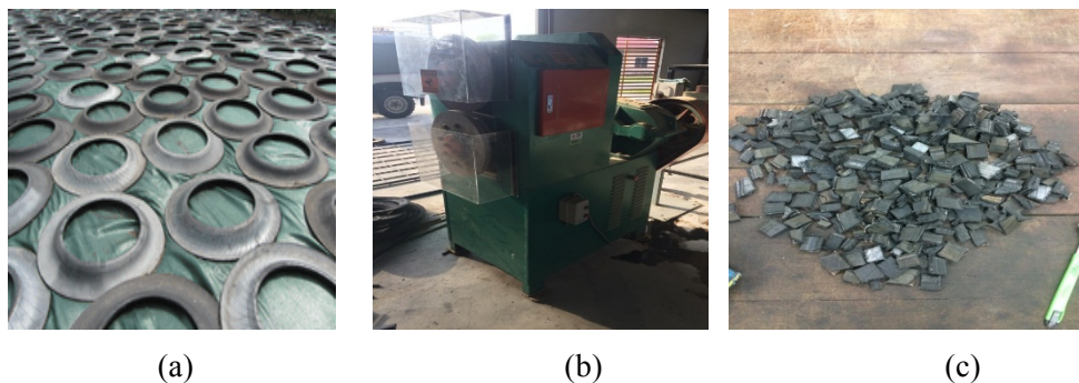
Figure 2. (a) tyre (b) shredding machine (c) crumb rubber.
