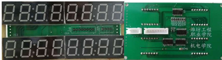
Figure 5. PCB of the display circuit
