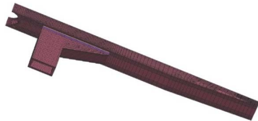
Figure 2. Assembly of side tube and connecting tube.
