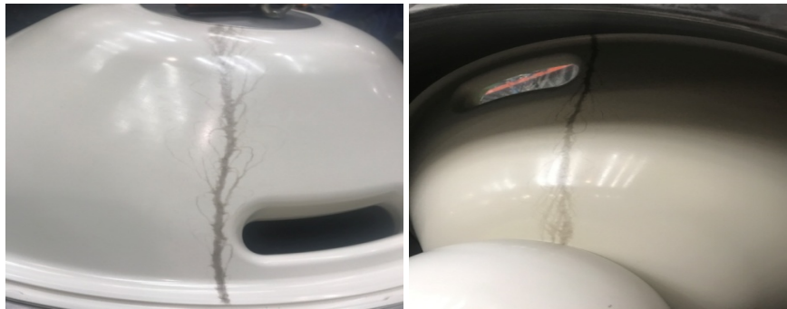
Figure 2. Basin insulator discharge trace
