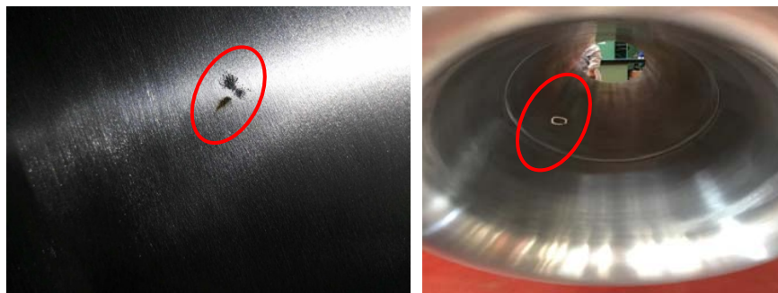
Fig.6 Shielding center conductor inner shield discharge photo
