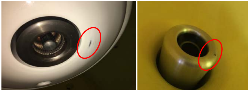
Fig.7 Grounding switch moving contact shield discharges the conductor shield
