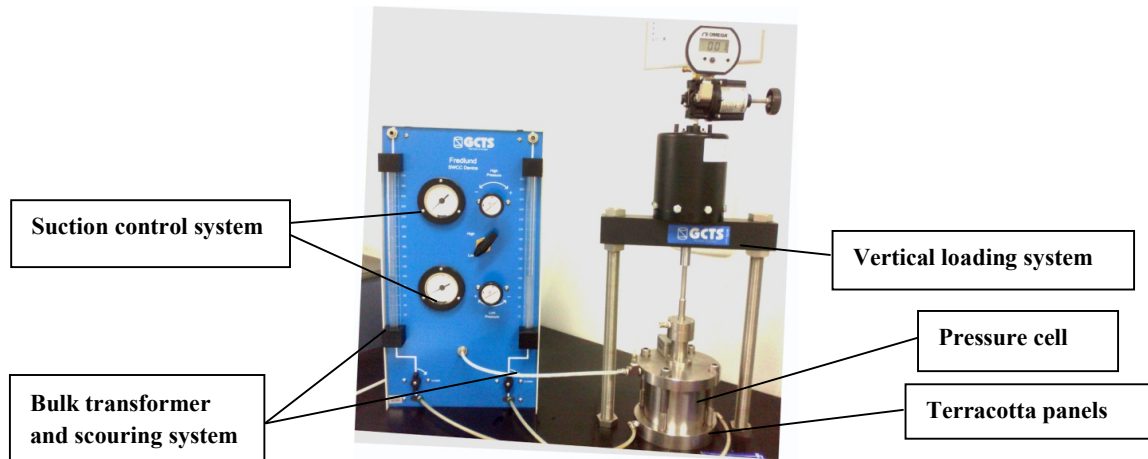
Figure 1. GCTS SWCC instrument photo.
