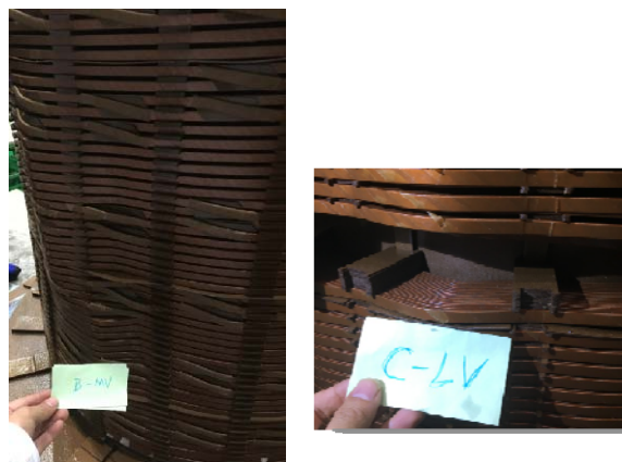
Fig.11 B-MV and C-LV winding deformation after short-circuit test
