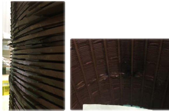
Fig.10 A-HV winding deformation after short-circuit test
