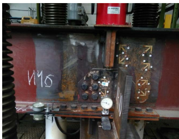
Figure 5. Model of a beam with combined half-end-plate and splice joint in the test bed.
