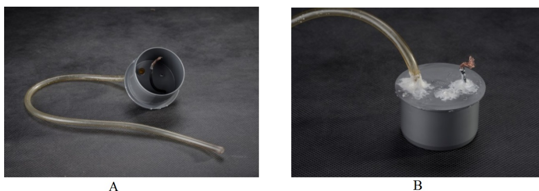
Figure 2. The cover of a single chamber BFC chamber with a gas discharge tube and a copper wire of 20 AWG OD (1.8 mm) for fixing the anode electrode. A - a view from the inside, B – a view from the outside
