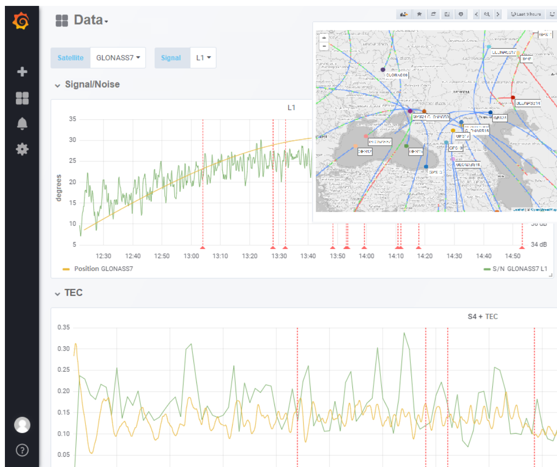
Figure 3. Ionospheric condition monitoring system according to the satellites' current location and trajectory.
