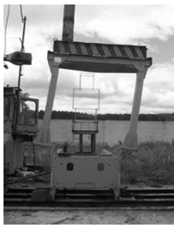
Figure 2. ROPS deformation under vertical loading.
