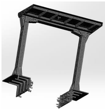
Figure 4. Model of boundary elements with mesh and snapping.
