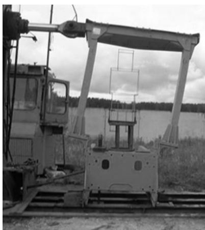
Figure 1. ROPS deformation under lateral loading.
