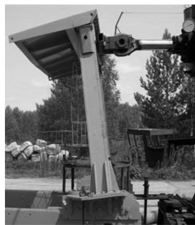
Figure 3. ROPS deformation under longitudinal loading.
