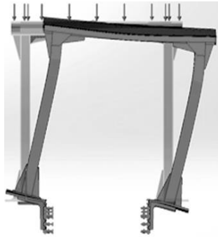
Figure 8. ROPS deformation under vertical loading.
