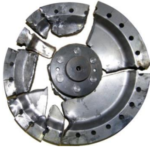
Figure 3. Photography of disc after burst
