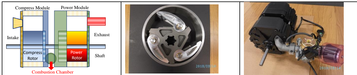
Figure 1. An eccentric swing blade rotary engine
