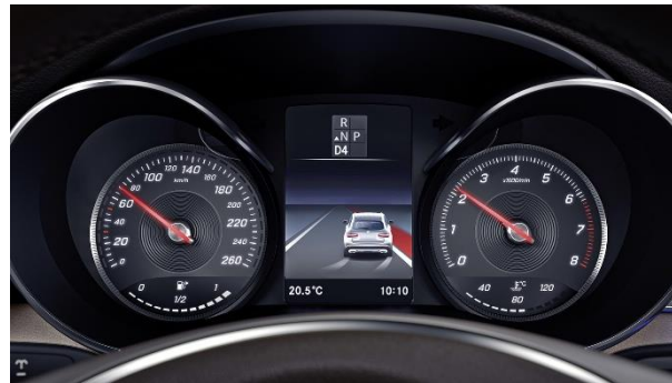
Fig. 6. Lane Keeping Assist show the traffic lanes in the Mercedes
