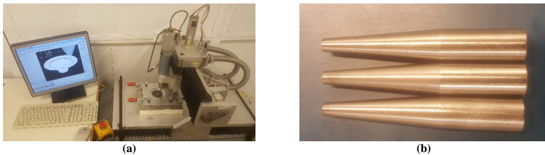
FIGURE 1. (a) Set-up of the experiments, (b) SPIF Tools with different corner radius
