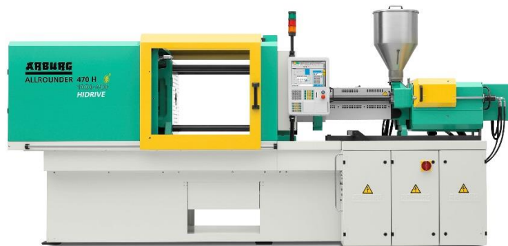
Figure 1. Arburg Allrounder 470 H injection moulding machine.
