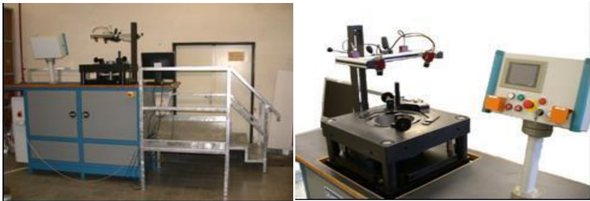
Figure 4. The Universal sheet metal formability testing system equipped with optical strain measurement system.
