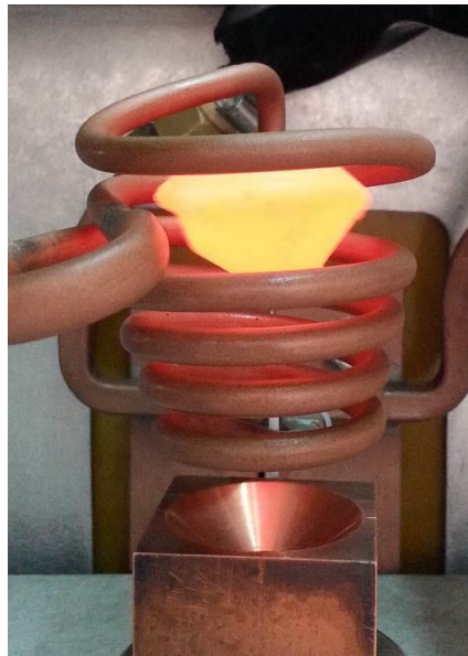
Figure 3. The Mg-Ca alloy button levitation melting inside the inductor.
