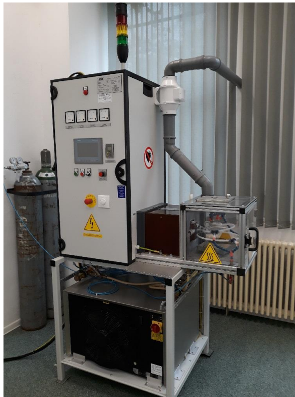
Figure 1. Levitation melter with medium frequency converter and inert atmosphere.
