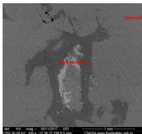
c) Segregation in central zone of sample 20
