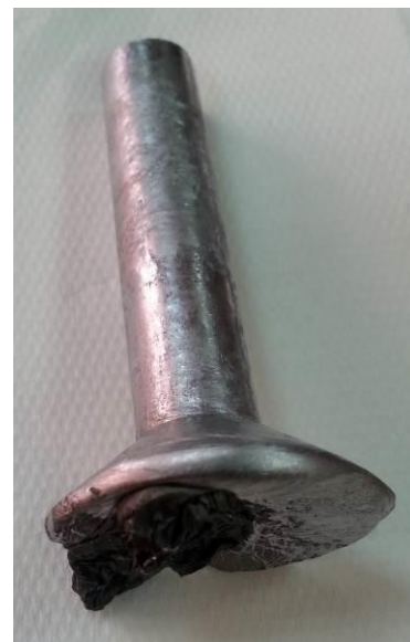
Figure 4. The appearance of the alloy during solidification and after extraction from the copper mould.
