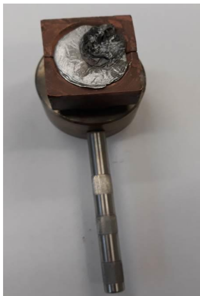
Figure 4. The appearance of the alloy during solidification and after extraction from the copper mould.
