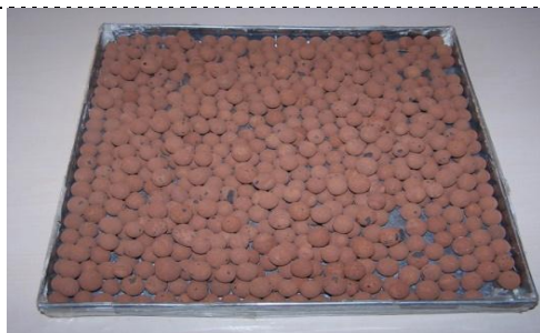
Figure 1. View of the class (12.5-16mm) of expanded clay granules
