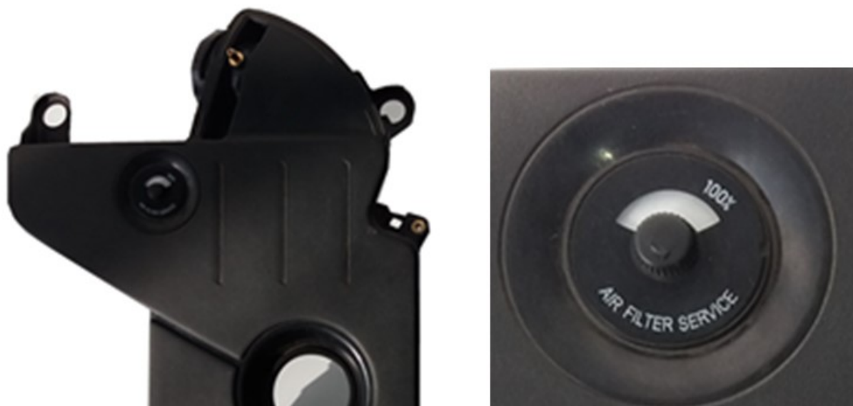
Figure 2. (a) Air filter housing equipped with air restriction indicator. (b) air filter “OK” (c) air filter replace
