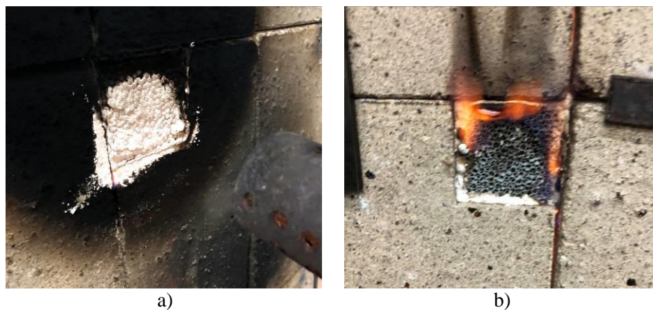
Figure 3. Aspects observed during the open flame test of sample 1: a) apparition of the intumescent layer on the anterior side, b) apparition of the open flame on the posterior side.
