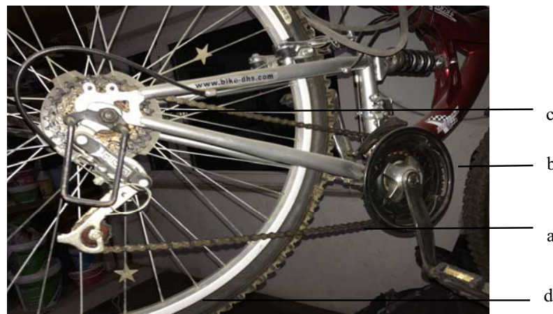
Figure 2. Chain transmission
