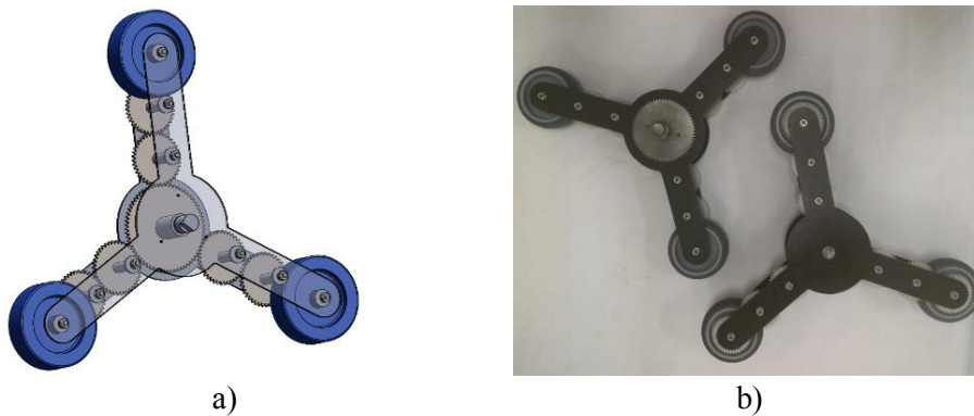
Figure 3. The 3D model a) and a photo b) of the locomotion unit.
