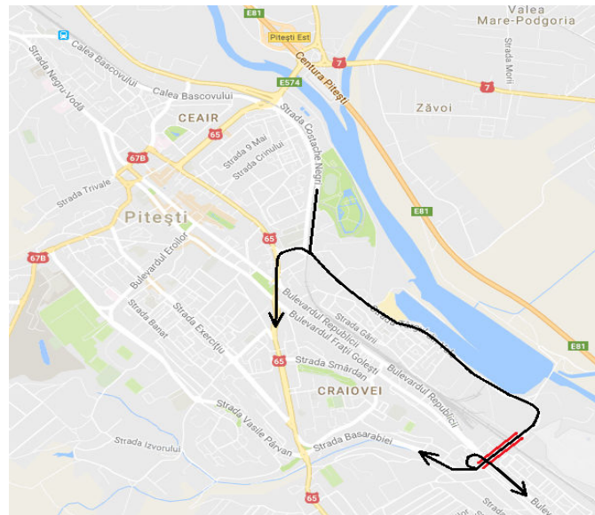
Figure 7. Redirecting part of the road traffic by arranging the Prundu passage [13].
