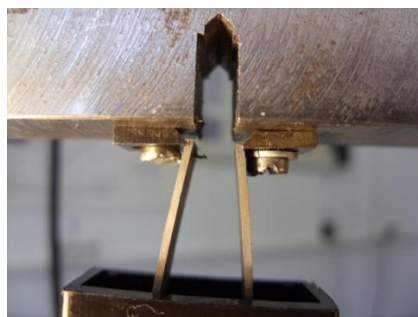
Figure 8. Mounting the extensometer.
