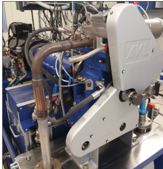
Figure 2. Compression ignition single cylinder engine mounted on single cylinder engine test bed.
