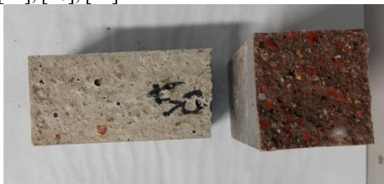
Figure 2. The utilization of fine RBA in fine aggregate concrete mixture (50% replacement rate)
