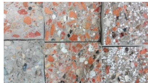
Figure 3. The utilization of coarse RBA in concrete mixture (up to 98% replacement rate)
