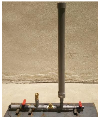
Figure 3. Hydram setup
