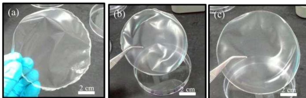
Figure 2. The produced film using (a) 0.50 g, (b) 0.75 g, and (c) 1.00 g of GG.
