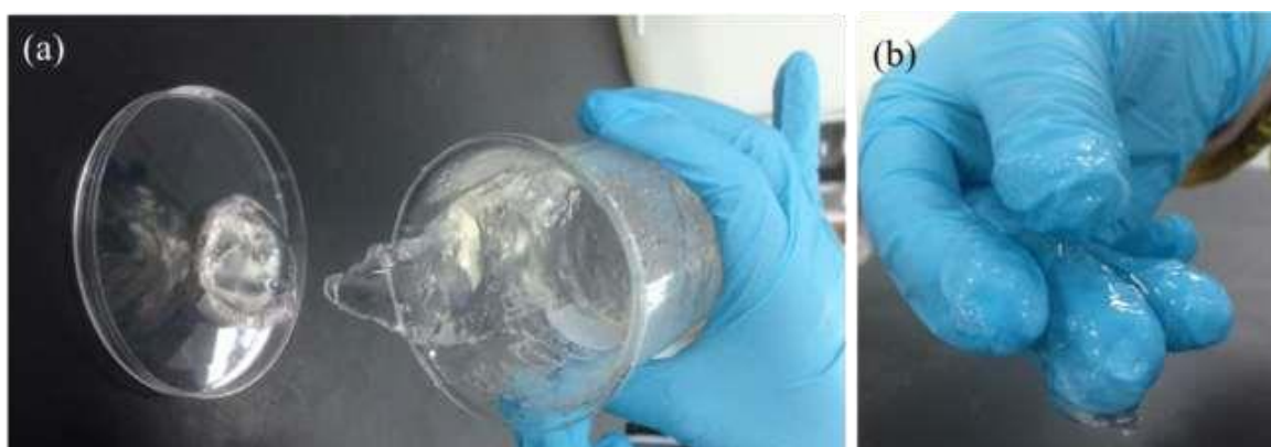
Figure 3. (a) Highly viscos, and (b) sticky GG suspension produced using 1.50 g GG.
