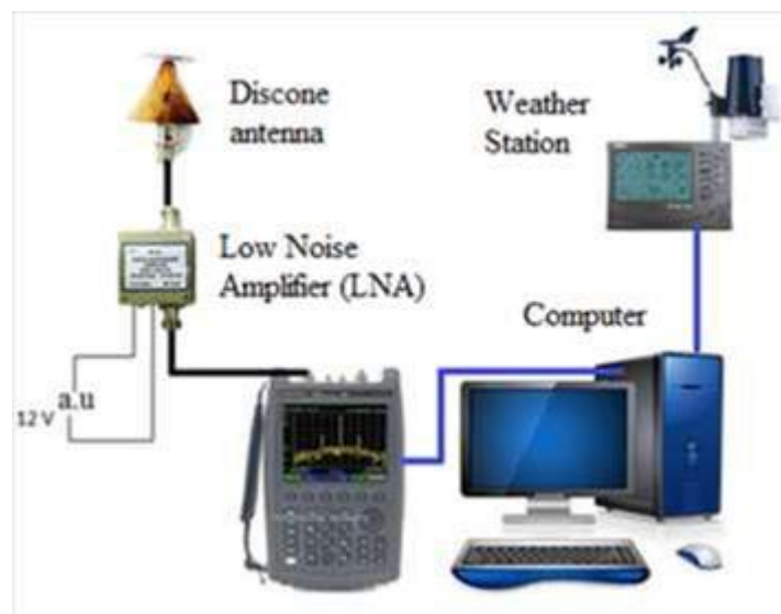
Figure 3. The instruments set up for observation work [5, 18-20]
