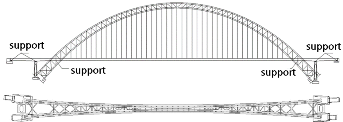
Figure 2-1. General layout of the long span half-through CFST arch bridge
