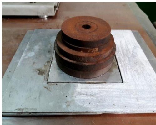
Figure 1. Post-stress applied during fabrication of composite.
