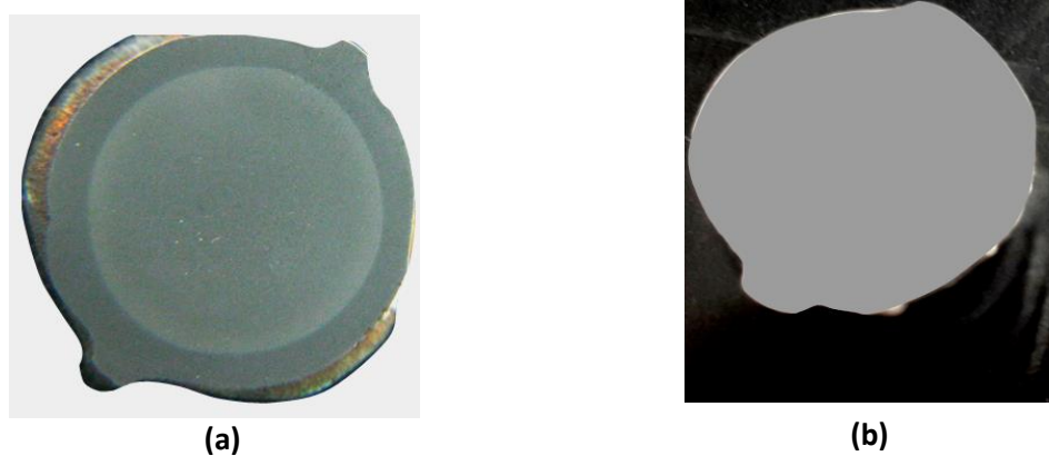
Figure 3. Macrophotographs showing etched surfaces of (a) 500MPa and (b) 300MPa bars.
