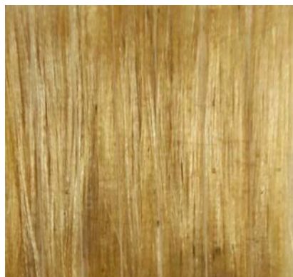
Figure 1. Jute-polyester composite.
