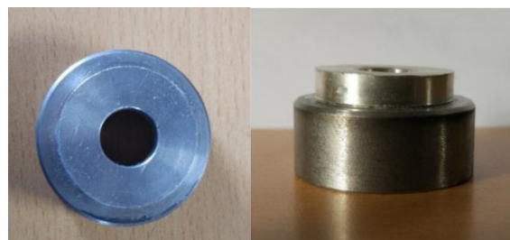
Figure 1. digital picture of the bonding strength test specimen
