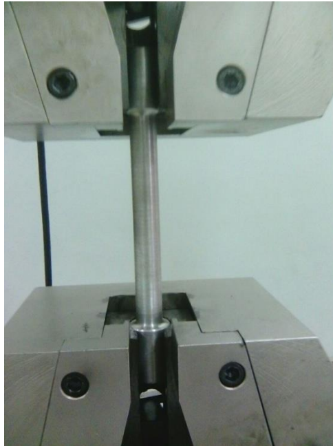
Figure 1. Specimen on universal testing machine.
