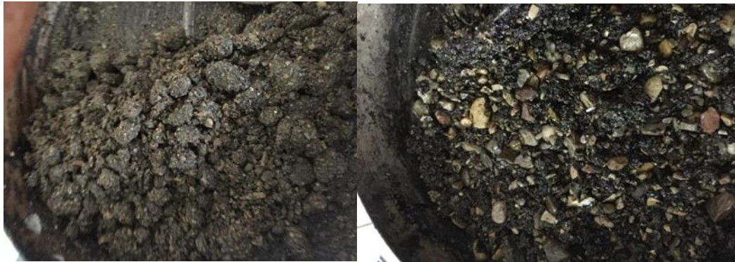
Plate 1. Compatibility and coating degree between different types of emulsified asphalt (cationic & anionic] with quartz aggregate.
