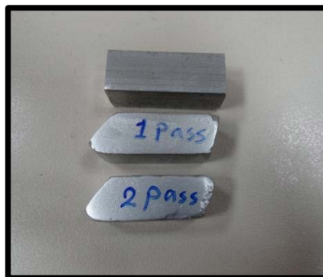
Figure 9. Billet shape after first and second passes.
