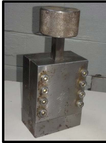
Figure 3. Die used to produce the billets
