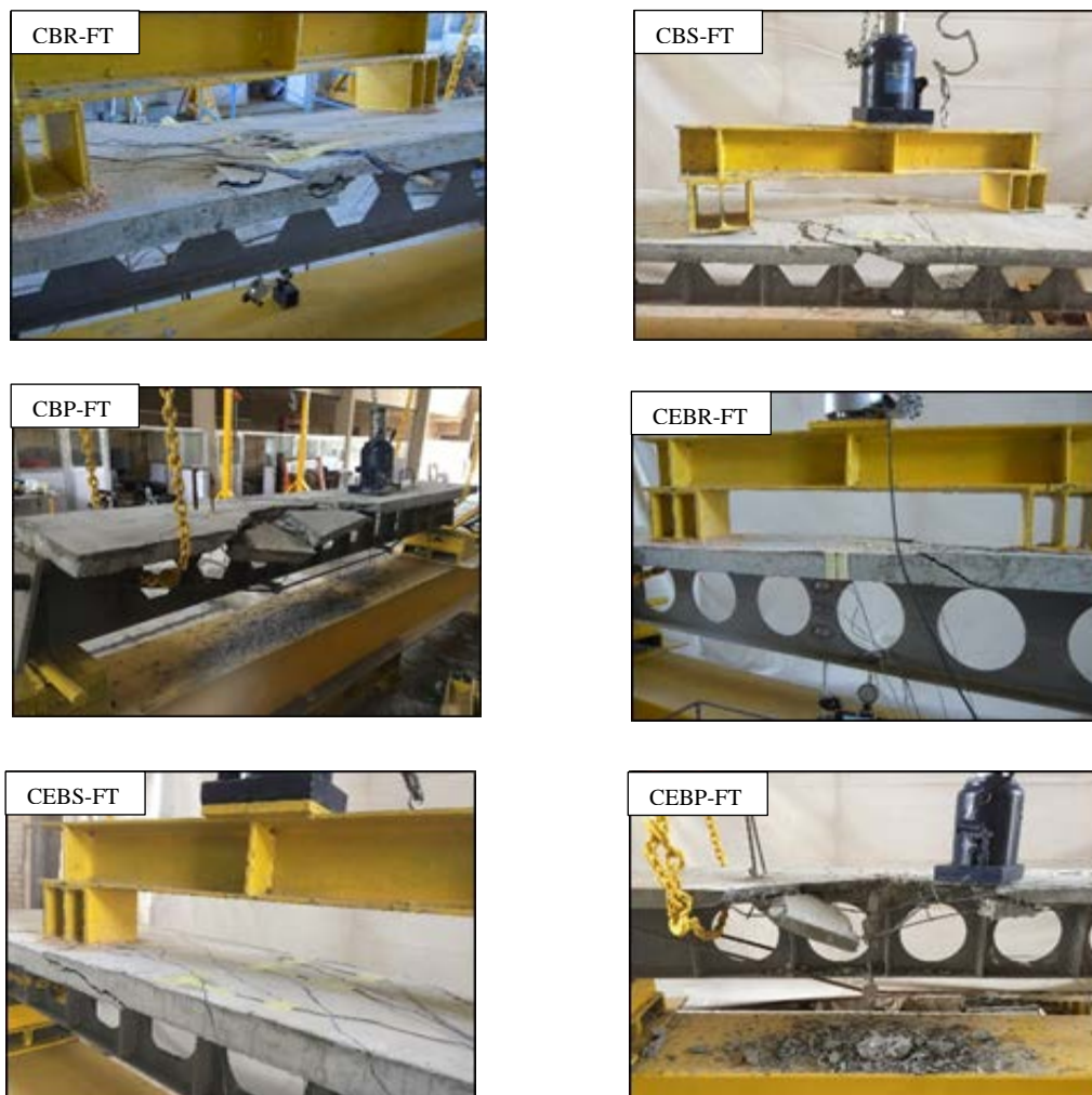
Plate 1. Modes of failure for experimental specimens [3].
