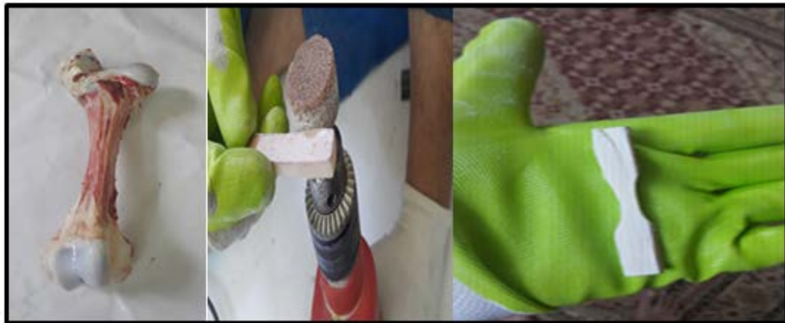
Figure 5. Cleaning the soft tissues from the femur bone and cutting rectangular specimens along the bone axis.
