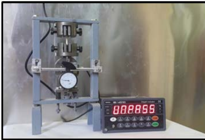
Figure 1. the Stress Relaxation Rig
