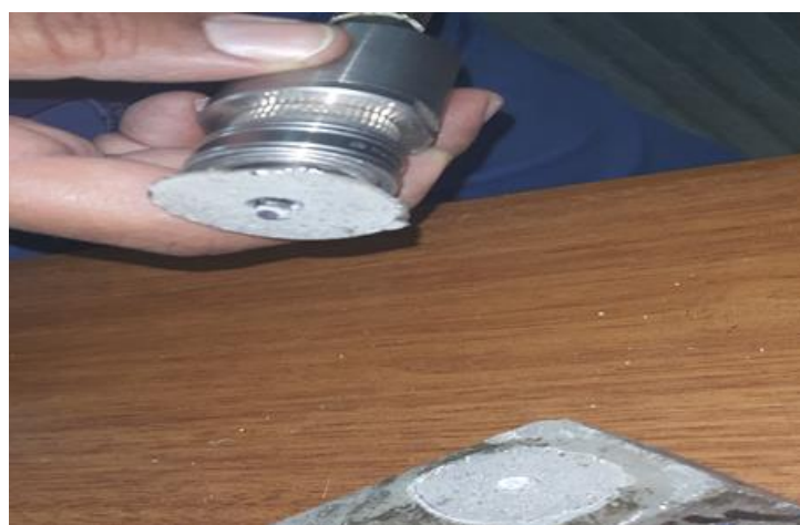
Figure (14) Dolly cohesive failure shown on the concrete substrate.
