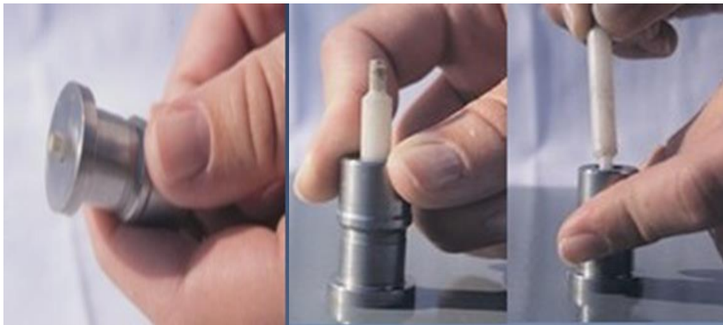
Figure (5) Measuring pull off adhesion using a type III (hydraulic) tester.
