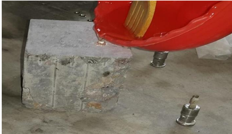
Figure (3) Sample of concrete specimens used in pull-off test.
