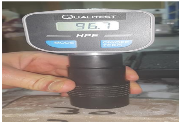
Figure (1) Digital durometer for Shore D hardness testing
