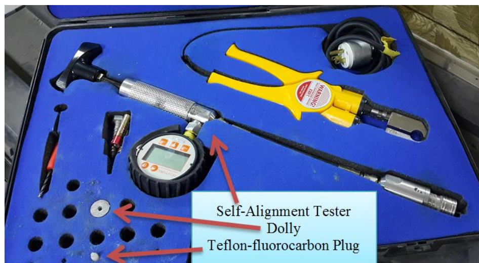
Figure (6) Actual equipment for Type III (Self-Alignment Tester) used in the pull-off test.
