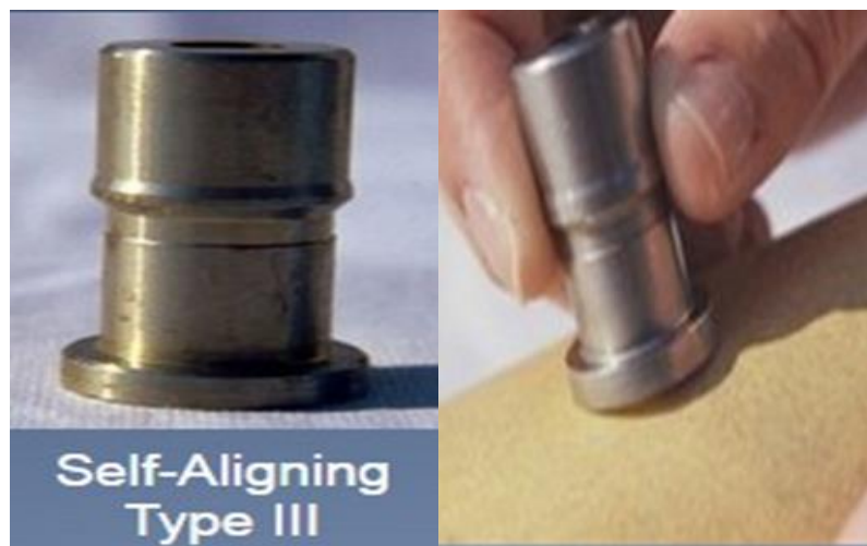
Figure (4) Self-aligning type III dolly [7]
