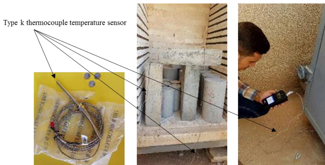
Figure 2. Measuring specimen temperature using an ELE thermometer.
