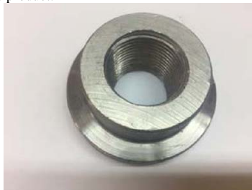
Figure 2. Gas cylinder neck sample
