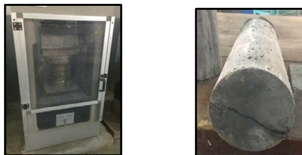
Plate 2. Specimen under machine and failure mode for splitting strength test
