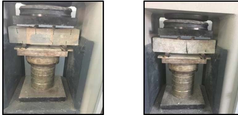
Plate 3. Specimen before and after test for flexural strength
