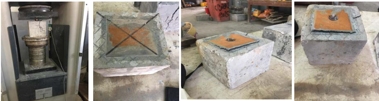
Plate 5. Cube specimens for reactive powder concrete with steel plate of 1 and 1.4 mm thickness at the top face of cube during and after test to determine the deformation constant k
