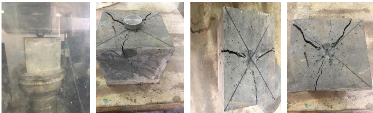
Plot4. Cube specimens for reactive powder concrete without steel plate during and after test to determine the deformation constant k
