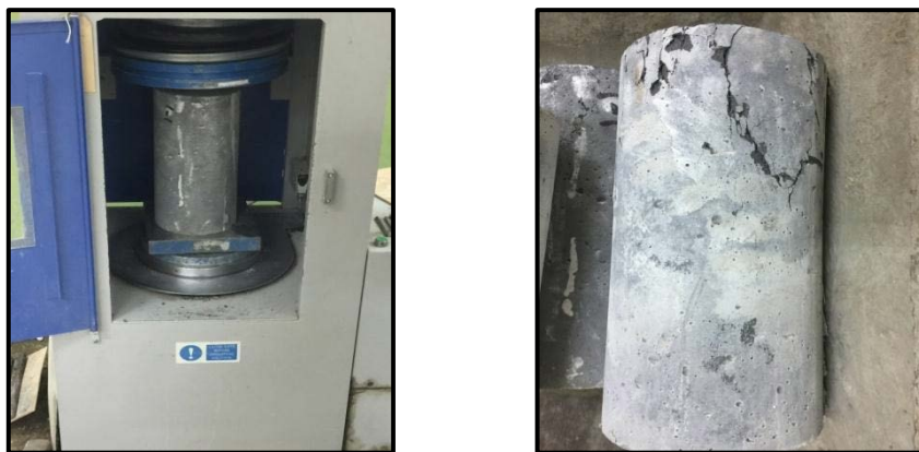
Plate 1. Specimen under machine and failure mode for compressive strength test
