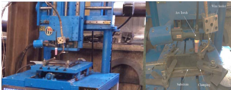
Figure 2 Left View of the CNC machine, and right side close-up view of the welding torch and filler wire nozzle
