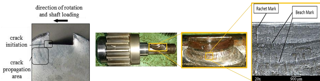
Figure 2. Direction of shaft loading.
